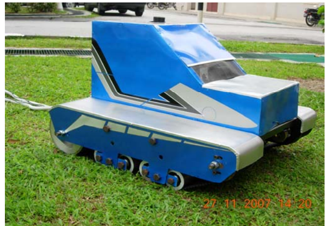
Fig. 6. Developed prototype of air-cushion track vehicle [9]
