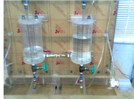
Fig. 1 The interactive coupled-tank process
