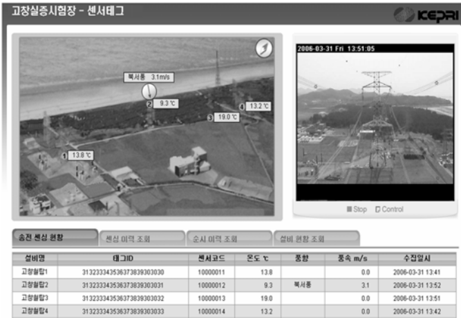
Fig. 5 Web screen of transmission tower monitoring system
