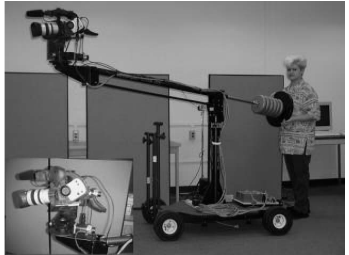
Fig. 1. The operator positions the camera by booming the arm horizontally and vertically. The pan-tilt head (inset) provides additional degrees-of-freedom.
