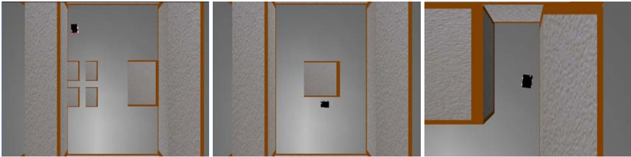
Fig. 8 Examples of environments in which the robustness of the visual contour following behaviour has been demonstrated: (left) with shortened obstacles that are not detected by ultrasound sensors; (center) obstacles with gaps; (right) square obstacle; and d) in a passage
