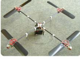
Fig. 1 Typical example of a quadrotor
