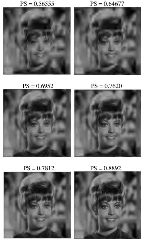
Fig. 10 “Zelda” image compression results. The images of the left column that follow are for SPIHT ONLY coded images. The images of the right column that follow are for the visually optimized SPIHT POEFIC coded images. The bit rates from top to bottom are 0.03125 bpp, 0.0625 bpp and 0.25 bpp respectively, at observation distance of V = 4
