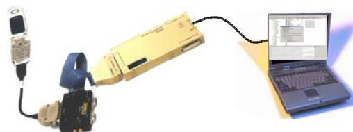
Fig. 2 Memory dump using JTAG
