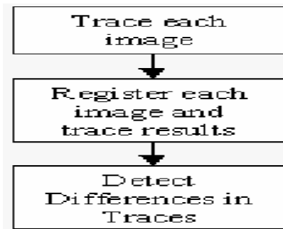
Fig. 1 Vessel change detection algorithm
