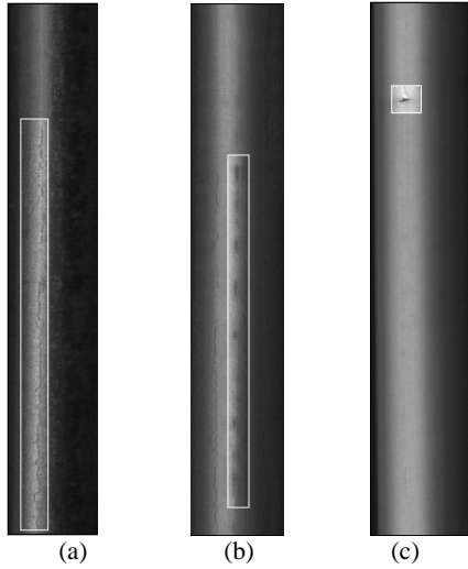
Fig. 1 BIC image (a) Crack (b) Dark line (c) Spot
