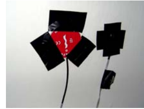
Fig. 5 Heat flux sensor and contact temperature probe
