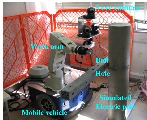
Fig. 1 Experimental power distribution line maintenance robot system
