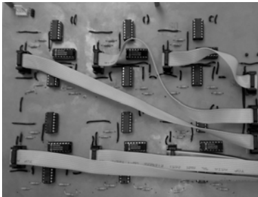
Fig. 2 Signal Conditioning Circuit
