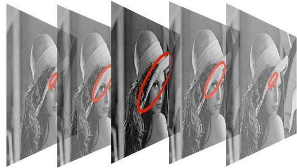
Fig. 3. Illustration of the idea of video steering kernel, here using five relatively identical frames. The third is the one we perform filtering on. The superimposed red ellipses represent level curves with same density of the kernel. It is obvious that redistributing some of the kernel weight on surrounding frames in this case can give a better estimate.
