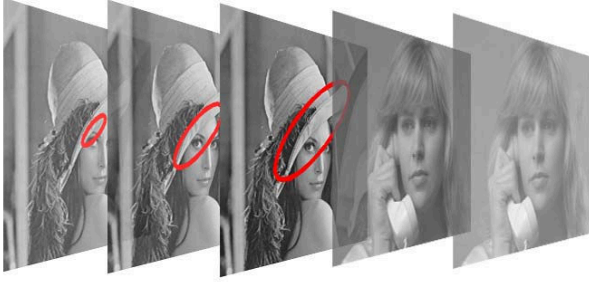
Fig. 4. Illustration of the idea of time asymmetric kernel, here using three relatively identical frames and a scene shift. The third is the one we perform filtering on. The superimposed red ellipses represent level curves with same density of the kernel. It is obvious that redistributing some of the kernel weight to frame 1 and 2 will give a better estimate, and that frame 4 and 5 should have little or zero weight
