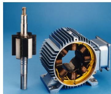
Fig. 1 A typical switched reluctance machine
