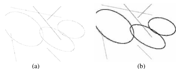
Fig. 3 (a) The synthesis ellipses with isolated noise, (b) The result superimposed on the image data.
