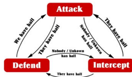
Fig. 8 Finite state machine to determine the team strategy
