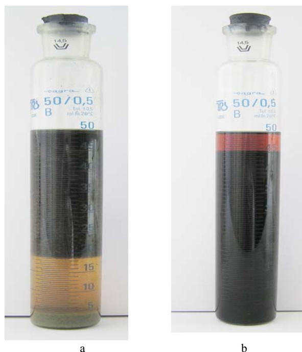
Fig. 2 Samples of liquid hydrocarbons that are obtained during aramide composite pyrolysis.
