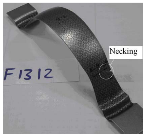
(b) 30×180 mm 2 sheet metal specimen
