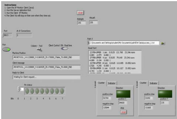
Fig. 2 Server for intermediate communicating between client and NC machine
