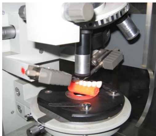
Fig.3. The method of laser micro spectral analysis is a method of punctual method of analysis, which allows to investigate small quantity of material, around 0.1 \mu\text{g} .
