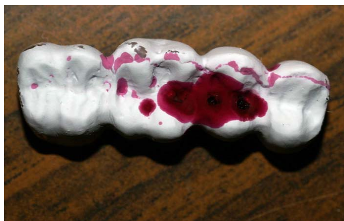
Fig. 2. The penetrating liquid method is used to point out the areas with material discontinuities.
