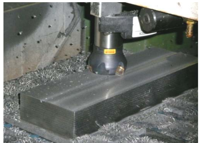
Fig. 2 Magnetic clamping of the workpieces
