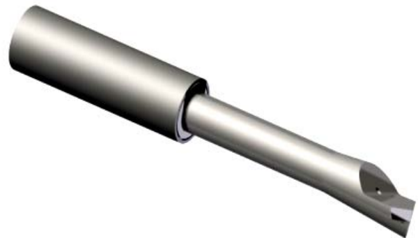
Fig. 5 CAD model of the boring bar
