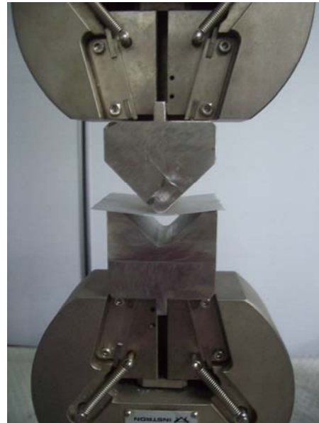
Fig. 2 Experimental set-up for V-bending process
