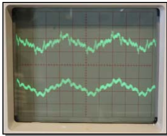
Fig. 6 Time domain plot of input (top) and output (bottom) of the DSK for circuit configuration in Fig. 5
