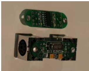
Fig. 5 Implemented and reprogrammed security hardware for PS/2 keyboard as an example. USB keyboard is not considerable for a secure keyboard because the USB host controller has no disposable interface between the host and the target device and it is adapted to the PS/2 interface through a combo converter
