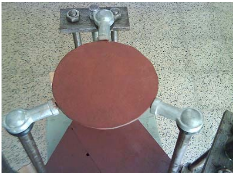
Fig. 2 A model of the 3 DOF Parallel Manipulator
