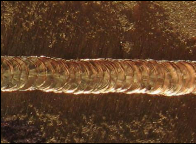
Fig. 1 Aspect of a welded Ni-Cr alloy sample (welding without filler): uniform overlapping of the spots, no visible defects
