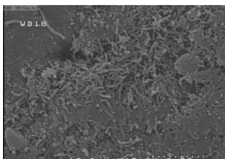
Fig. 17 FE-SEM image of Al-CNT composite after compaction
