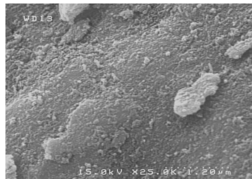
Fig. 12 The FE-SEM image of Al-MWCNT after the mixing process
