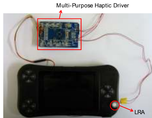
Fig. 4 The implemented system for the authoring tool
