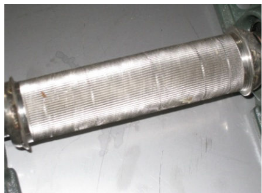
Fig. 11 The transmission shaft conveyor
