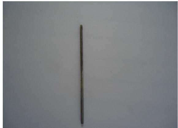
Fig. 2 Stainless Steel tool (diameter : 0.7mm)
