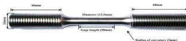
Fig. 2 Test specimen shape and dimension (KS B0801 10)
