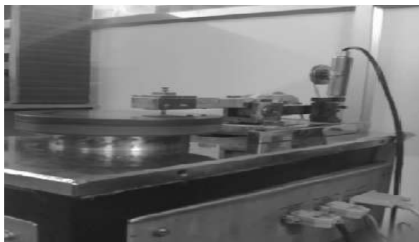
Fig. 2 Experimental Setup for Wear Testing
