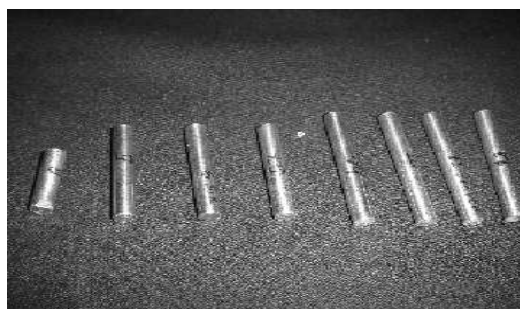
Fig. 1 DMLS Wear Testing Specimens
