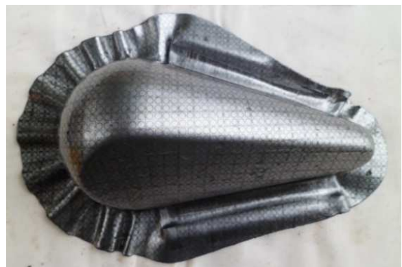
Fig. 12 Workpiece with grid to measure the strain
