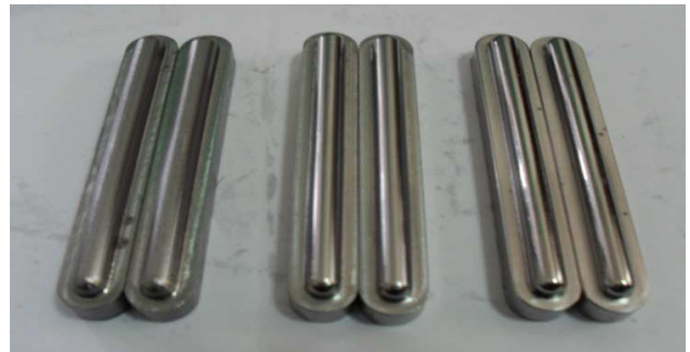
Fig. 4 Drawbeads with 3 levels of surface roughness from left to right: 6.127 \mu\text{m Ra} , 0.963 \mu\text{m Ra} , and 0.152 \mu\text{m Ra}
