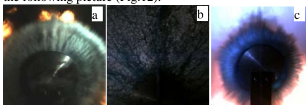
Fig. 12 Several patterns of liquid explosive dispersing flow. a: Inertial dispersion; b: Turbulent dispersion; c: Mixture of inertial and turbulent dispersion
