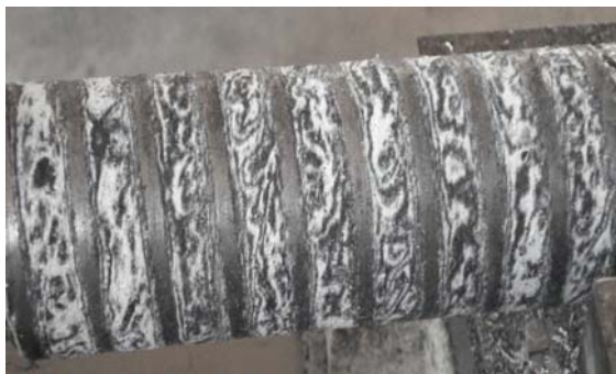
Fig. 3 Fibers wound on the mandrel
