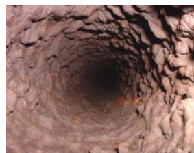
Fig. 17 Different cases of internal corrosion in metallic water pipes
