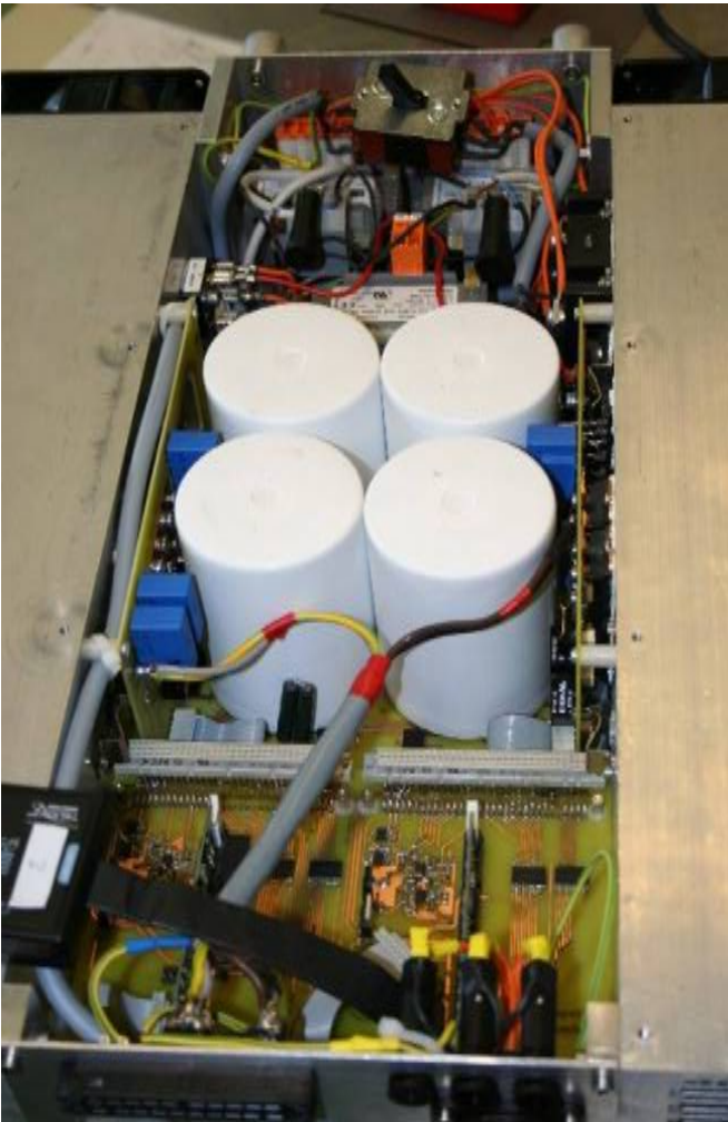
Fig. 6. Insight into a hot swap controller amplifier module prototype: digital signal controller section with digital signal control-cards (Texas Instruments TMS320F28335) on the lower side; power stage with 25 kVA in the centre and low level power supply transformers (400Vac to 230Vac) and mains switch on the upper side.
