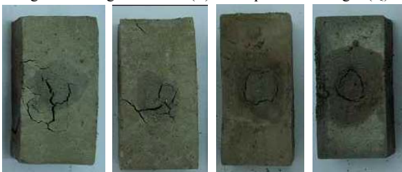
Non-baked specimens: severely damaged during tests
