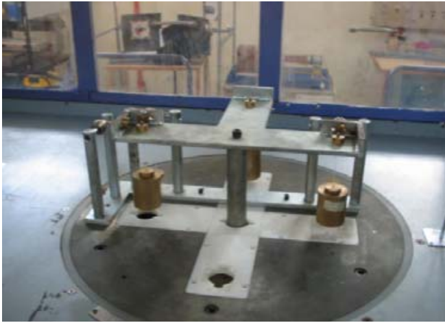
Fig.3. Calibration rig mounted on the floor of the wind tunnel test section
