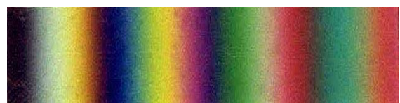
Fig. 8 The photoelastic color sequence
