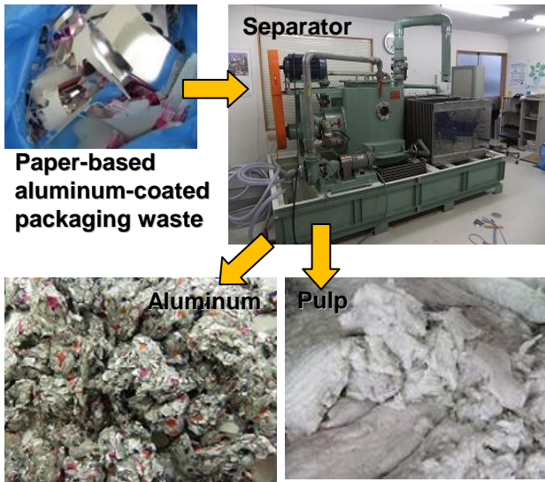
Fig. 4 Paper-Aluminum separation process
