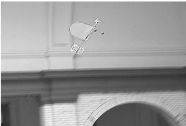
Fig. 4. Fixed-wing prototype prop hanging with a large angle-of-attack
