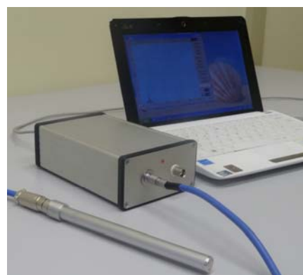
Fig. 2 The dosimetry system: the detector, the Flip-flop electrometer, a computer with the DoseX ® software
