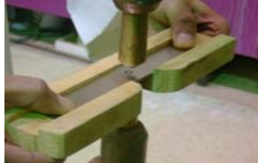
Fig 2 Spot welding specimen holder
